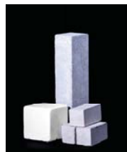
ABOVE: MCI product prototypes, plasterboard and concrete: produced via mineral carbonation at the MCI Pilot Plant in Newcastle.
