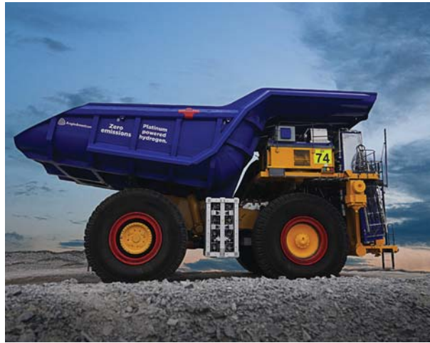
ABOVE: The nuGen Zero Emission Haulage Solution is a hydrogen-powered ultra-class mine haul truck from Anglo American, said to be the world's lightest 510 t truck.
