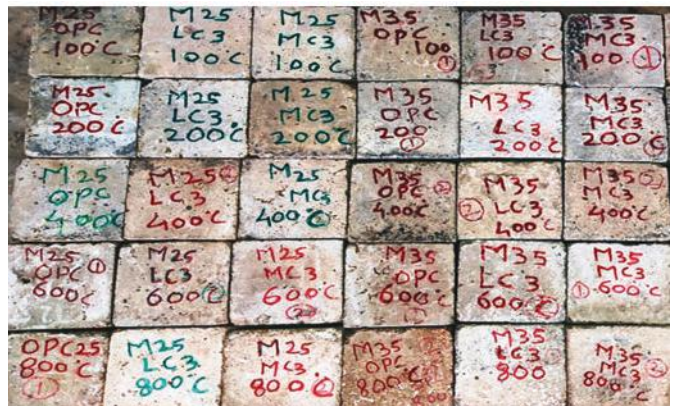
BELOW RIGHT: Cracks occurred in M25 OPC, LC 3 and MC 3 concrete specimens.
