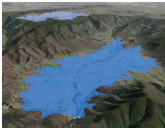
LEFT: Class AA 500 GWh site near Araluen in Australia, with a head of 600 m.
