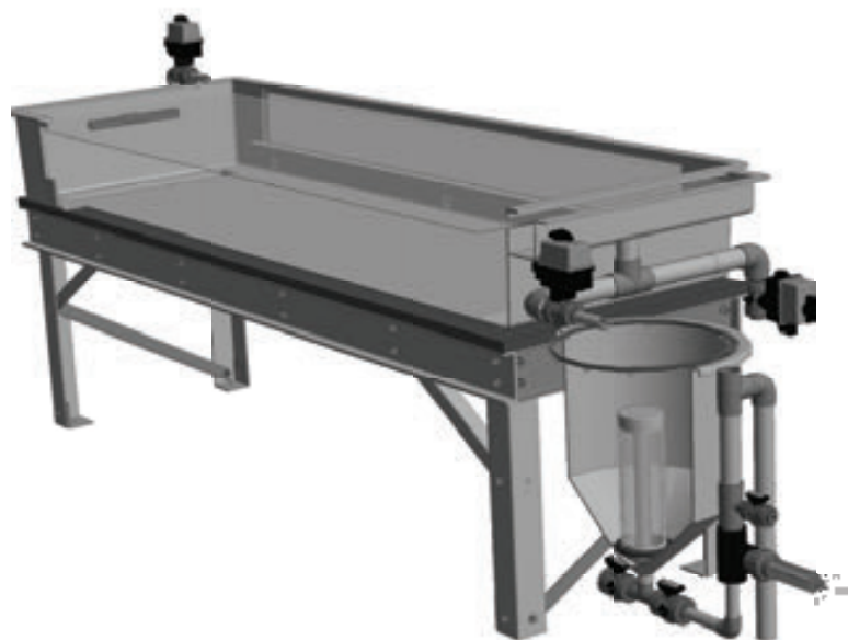
RIGHT: The coral spawning system automatically harvests egg/sperm bundles and manages the fertilisation process using auto valves and feedback from turbidity sensors.
