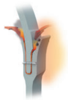
An exaggerated diagram of the joint rotation that enabled combustion gas to pass through the field joint.
